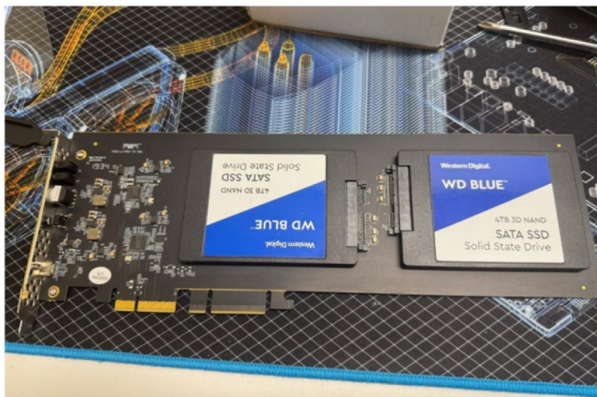
Some PCIe cards, such as this Sonnet Fusion card with two WD Blue SSDs, must be used in specific PCIe slots.
