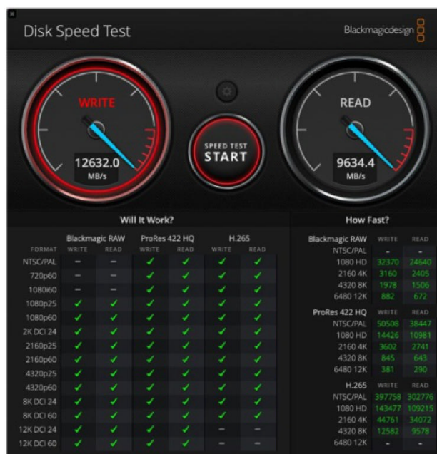
Blackmagicdesign's Disk Speed Test benchmark of four Samsung 970 EVO Plus NVMe SSDs in a Raid 0 array on a Sonnet PCIe card.
